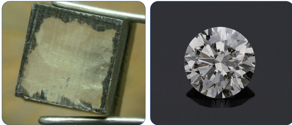
[A10mm single crystal diamond substrate(left), 1.27ct brilliant cut diamond(right)]
